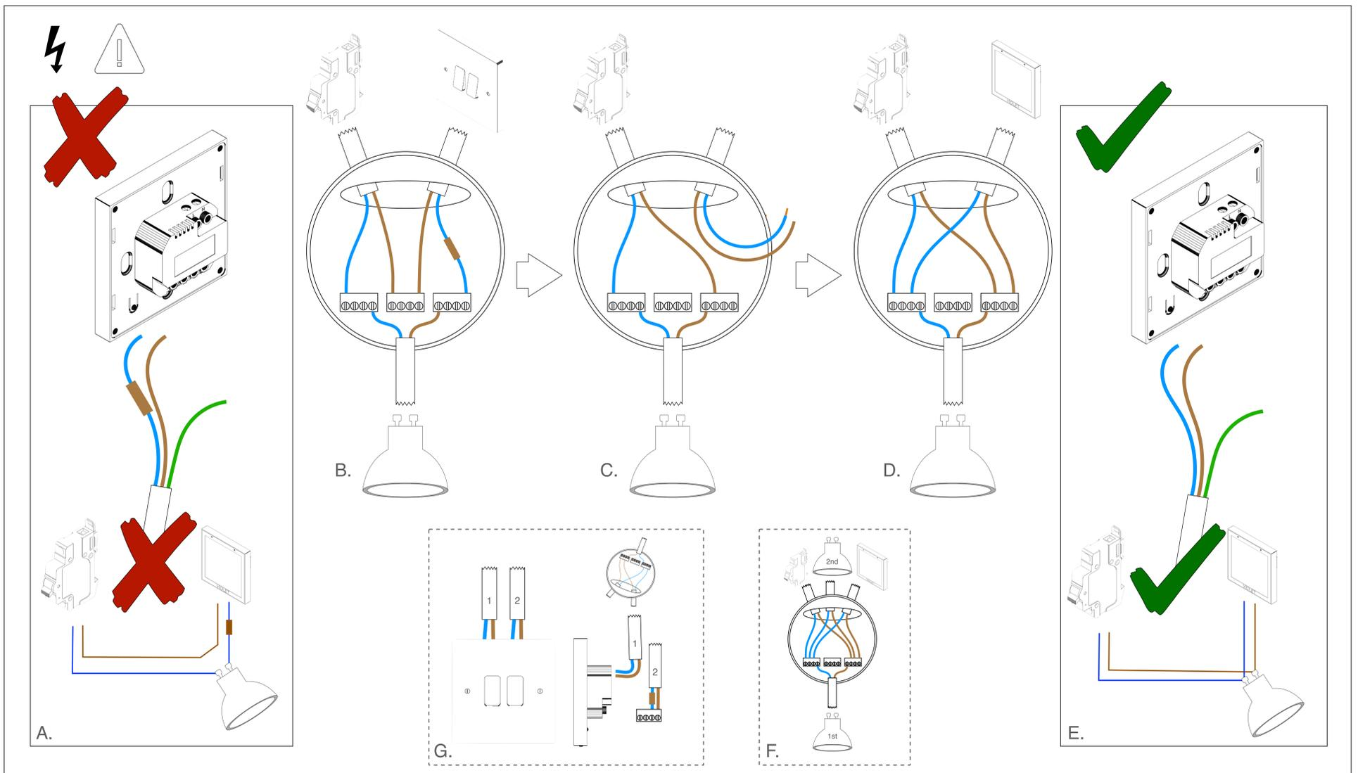
Some homes will not have a neutral at the switch location (A), they have a switched-live (usually marked with brown tape). Since SmartSwitch Lite requires a neutral, there is a small change that needs to be made to utilise the existing wiring. **[Note: If you do have a neutral at the switch location already (very likely in mainland Europe), then the same concept discussed below applies just at the switch itself rather than the light location.]**
