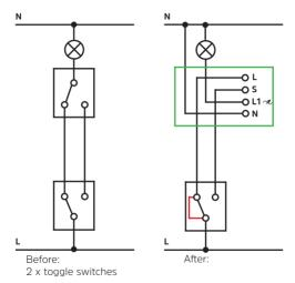
The existing toggle switch must be bridged out in this connection example.
