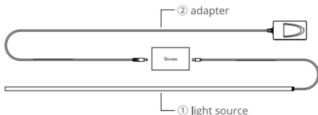
The product is divided into two parts: (1) a light source and (2) an adapter. By detaching the output terminal of the adapter, you can easily remove the light source or the adapter.
