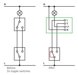
The existing toggle switch must be bridged in this connection example.
